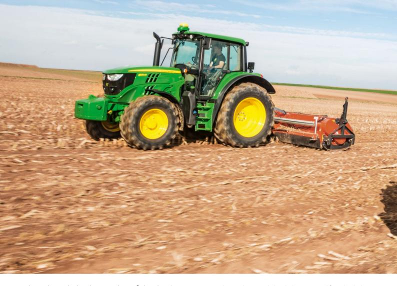
The acknowledged versatility of the 6M Series is complemented by our available hitches, drawbars and PTOs and enhanced by the convenience of ISOBUS connectivity with a wide range of productive implements. The new rear hitch is identical with that on our premium 6R tractors, and delivers the same maximum lift capacity of 8500 kg. Available PTO speed options are 540/1000 rpm or 540/540E/1000 rpm.
