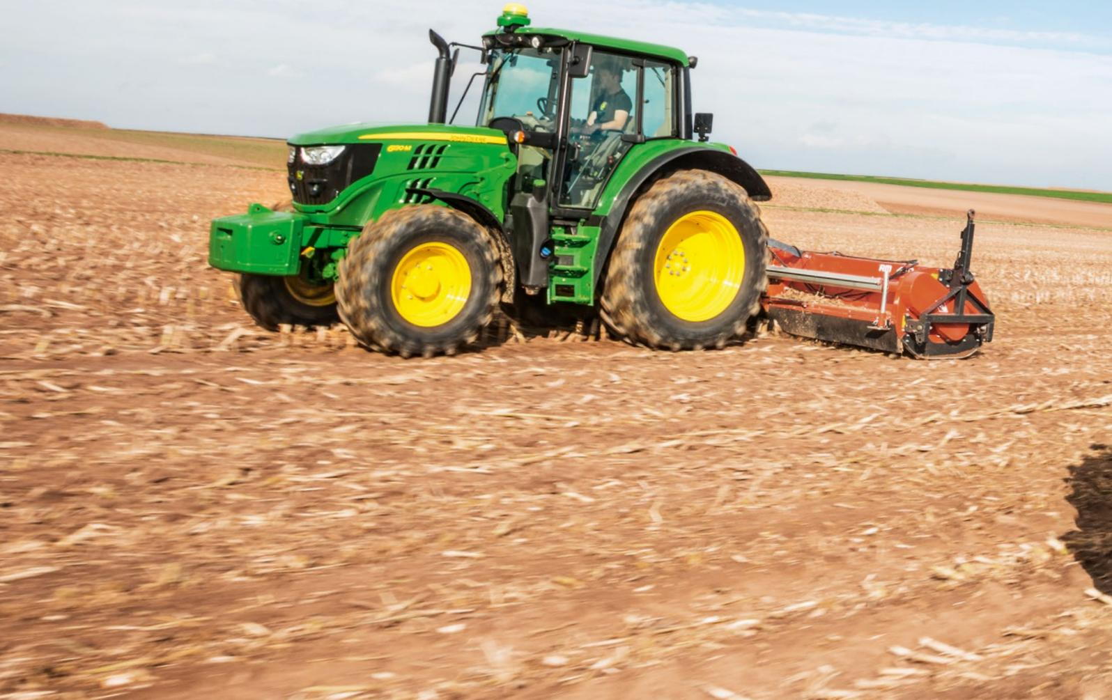
The acknowledged versatility of the 6M Series is complemented by our available hitches, drawbars and PTOs and enhanced by the convenience of ISOBUS connectivity with a wide range of productive implements. The new rear hitch is identical with that on our premium 6R tractors, and delivers the same maximum lift capacity of 8500 kg. Available PTO speed options are 540/1000 rpm or 540/540E/1000 rpm.
